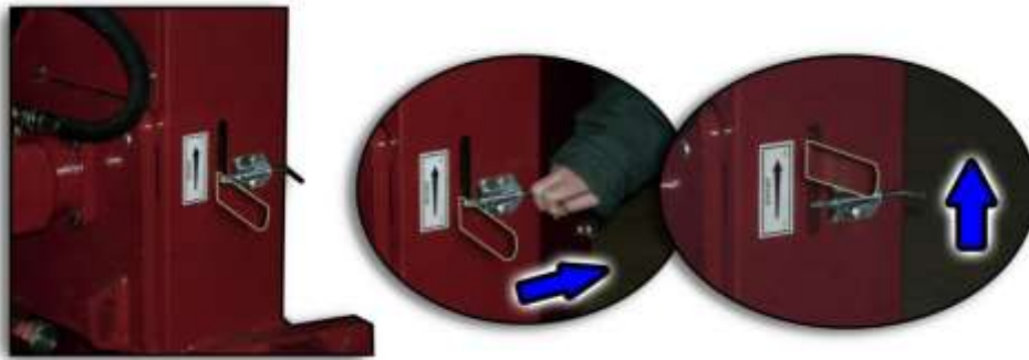
Figure 9 - Engage Brake Prior to Transport
