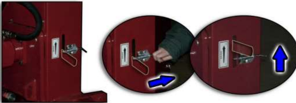
Figure 18 - Engage Brake Prior to Transport
