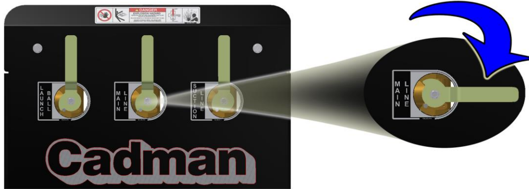
Figure 12 – Main Line Valve – Turn to VENT Position
