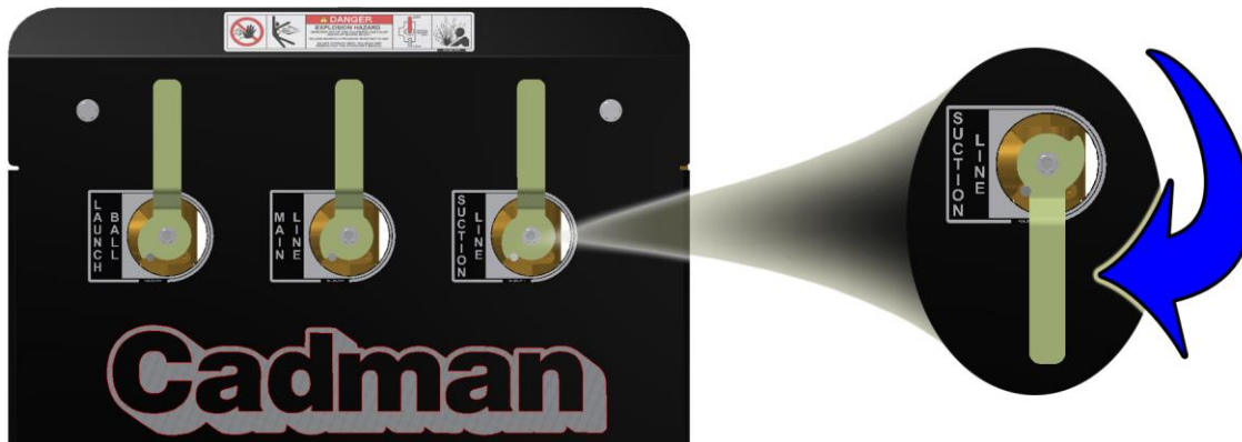
Figure 14 - Suction Line – Turn to PURGE Position
