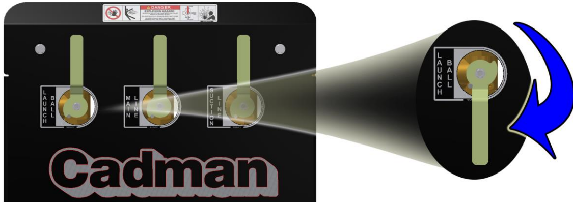
Figure 11 - Launch Ball Valve – Turn to PURGE Position
