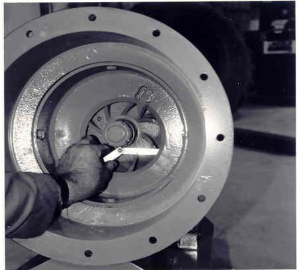
**NOTE:** Impeller plate hole is offset to the lower right.
