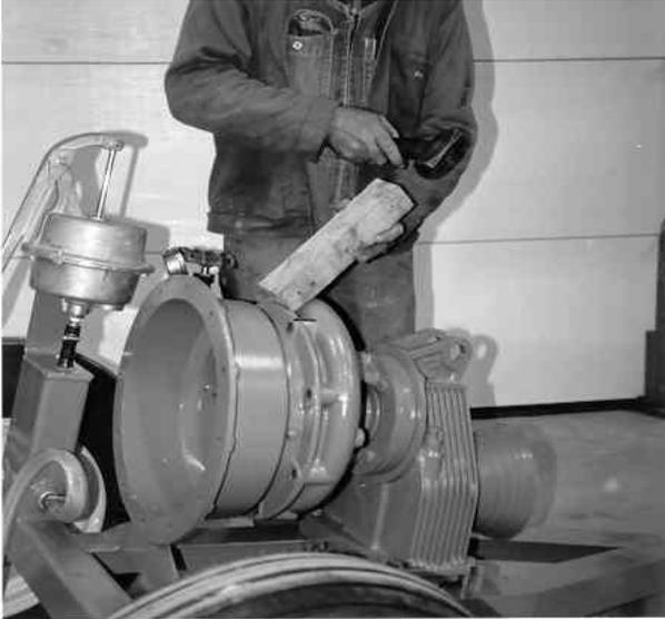
4. Using a block and hammer, carefully work around the volute extension until the two pieces separate. The impeller cover should be left attached to the volute extension
