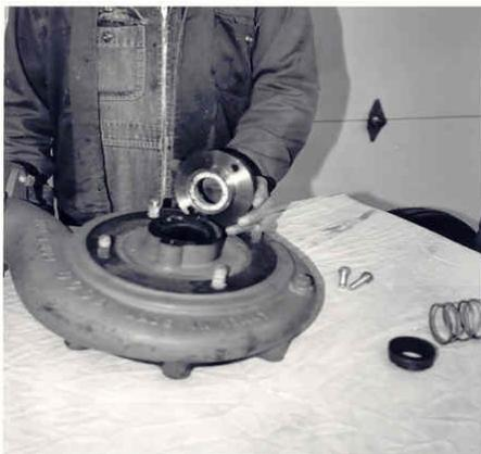
9. Remove the glad plate from the volute. Remove the impeller nut.
