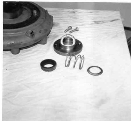
10. Old seal components are stationary seal face (A), rotating seal face (B), spring and spring washer. Remove the glad plate from the volute. Remove the impeller nut.
