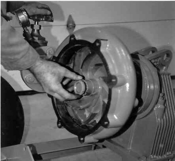
6. Remove the impeller nut.
