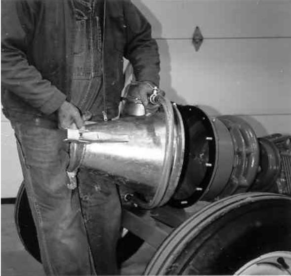
1. Remove the suction cone from the volute extension. The suction hose to the hand primer may be left attached if care is taken not to damage the hose.
