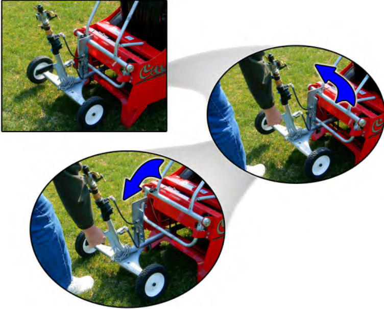
Figure 14 - Lower Sprinkler Cart
