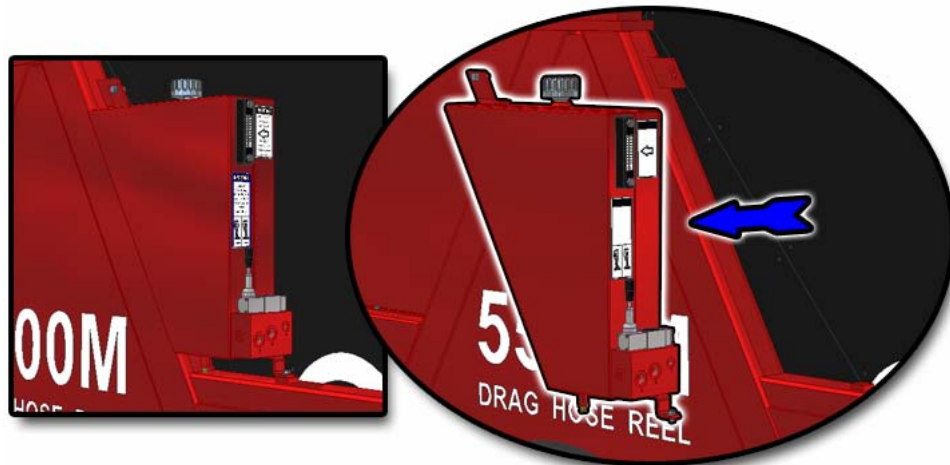
Figure 9 - Remove Hydraulic Tank
