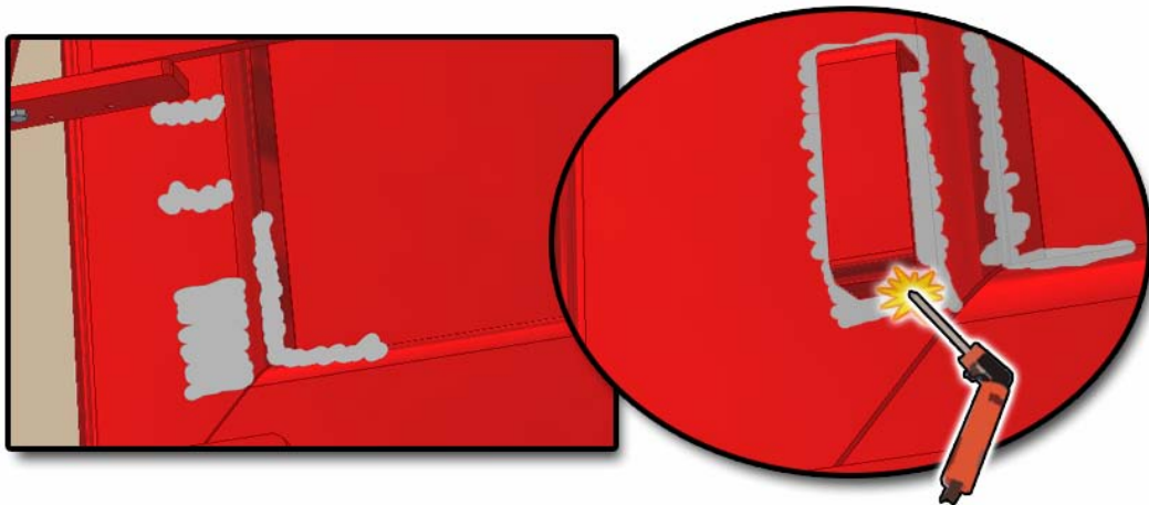
Figure 16 - Weld hose guide in new Location
