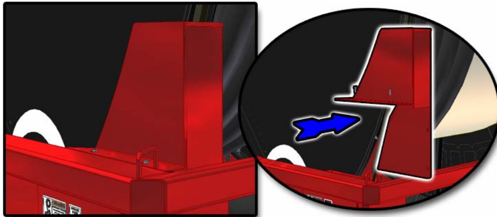
Figure 27 - Remove Front Chain Guards
