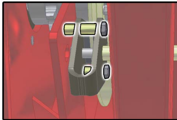
Figure 52 - Install Brake Caliper Bolts and Spacers
