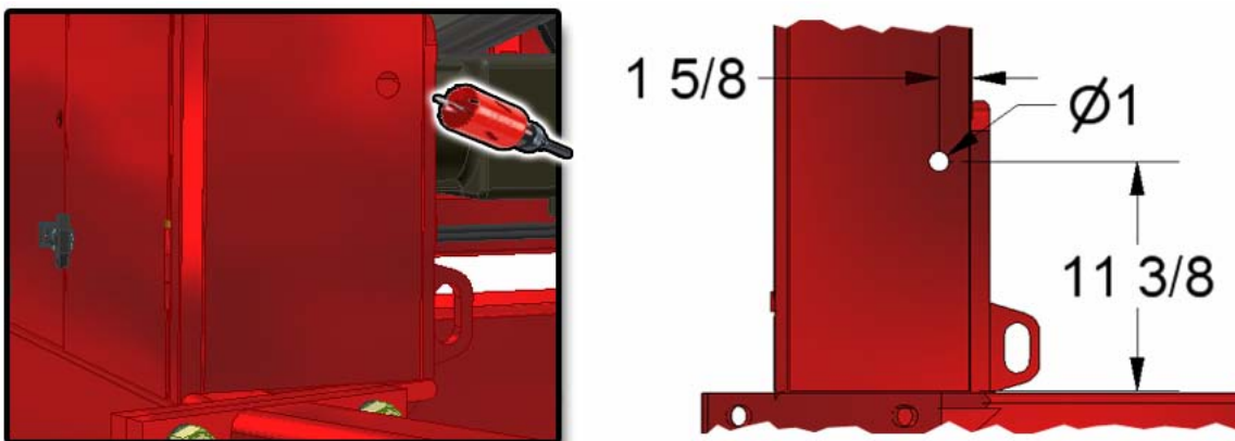
Figure 38 - Cut Greasing Access Hole
