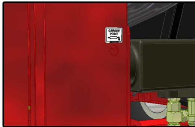
Figure 54 - Install Grease Point Label
