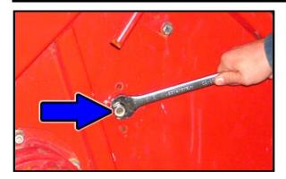
Remove stationary idler sprocket.
