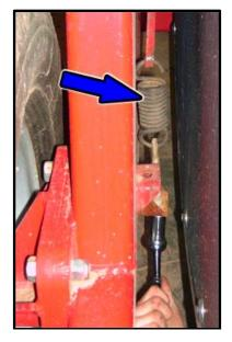
Re-install chain tensioner spring and tighten nut with a ratchet wrench until proper tension is achieved.
