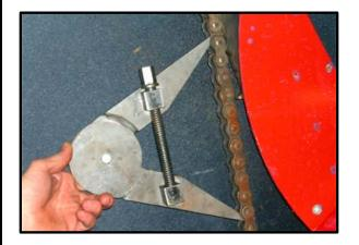
Using a chain whale, connect the chain ends re-using the master link.
