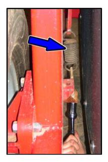
Remove chain tensioner spring by slowly loosening nut with ratchet wrench.
