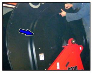
Install the new chain guard included in the upgrade package.
