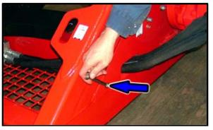
Remove 5 bolts. Remove side shield.
