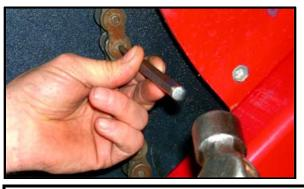
Use a punch to remove cut link.
