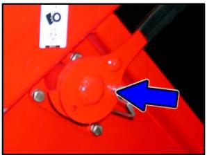
Install drum lock handle with 3 bolts.
