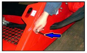
Remove 5 bolts. Remove side shield.
