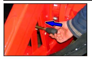
Re-install brake handle and tighten to prevent drum rotation.
