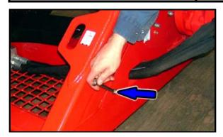
Engage drum lock, remove brake handle, reinstall side shield and brake handle.
