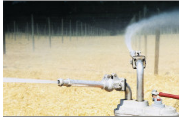
Asymmetrical Broadcast Cart in operation at a ginseng farm.
