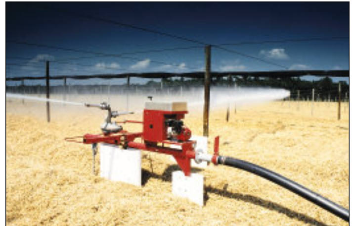
Asymmetrical Broadcast Cart in operation at a ginseng farm.
