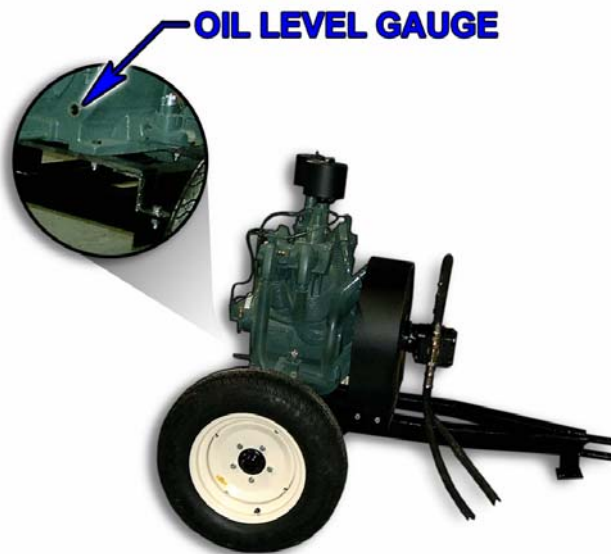
Figure 2 - Compressor Oil Level Gauge
