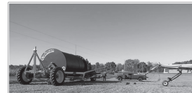
The hose guide can raise 4' above the ground keeping the hard hose from dragging over crops.
