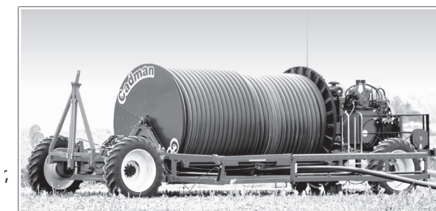
The CMA automatically moves ahead when the tractor turns to start another row.
