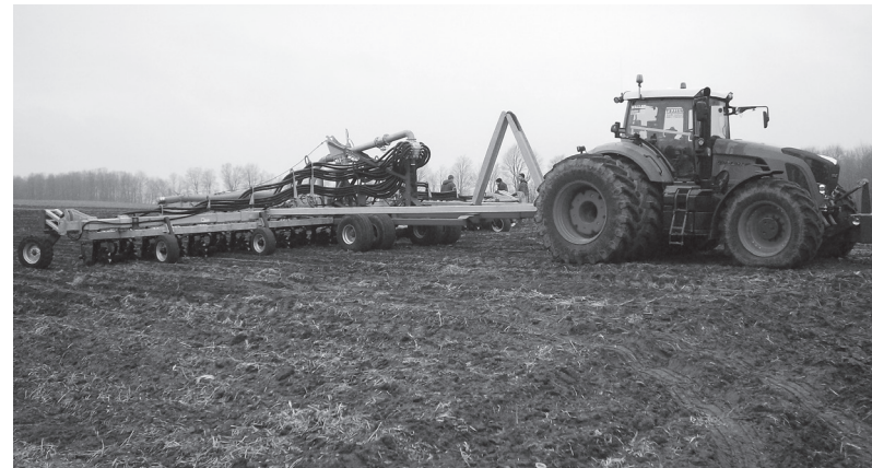
40' Injector with VTI tooling.
