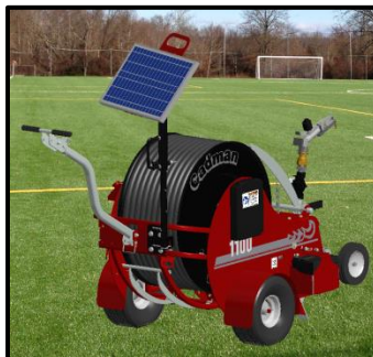
Figure 33 - Solar Panel Assembly Completed
