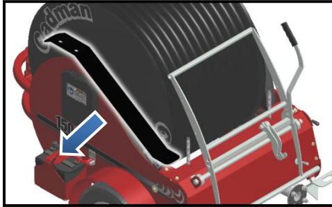
Figure 36 - Remove Chain Guard
