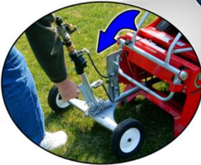
Figure 13 - Lower Sprinkler Cart
