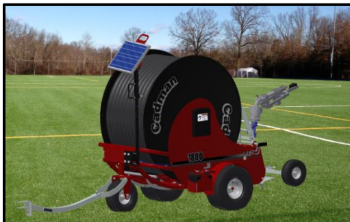
Figure 33 - Solar Panel Assembly Completed
