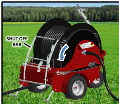
Figure 25 - Verify Shut-off System
