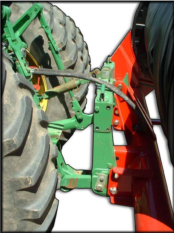
Figure 3 - Connect to caddy with 3-Point Hitch (Quick Hitch System shown)
