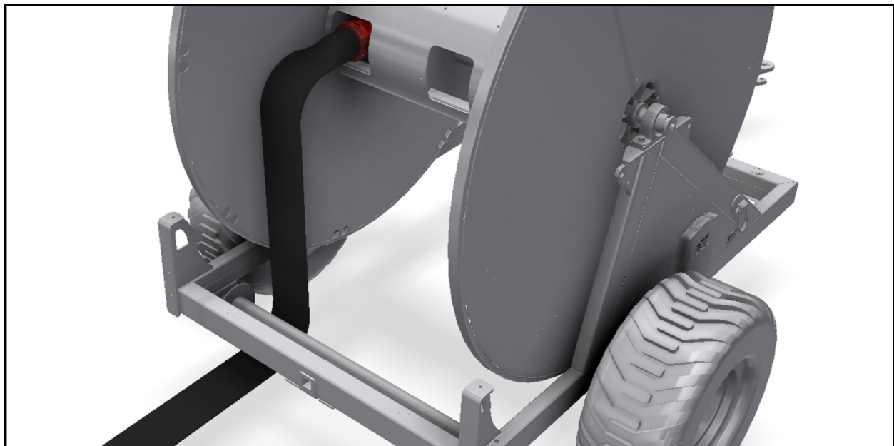
Figure 15 - Insert Hose into Reel Opening
