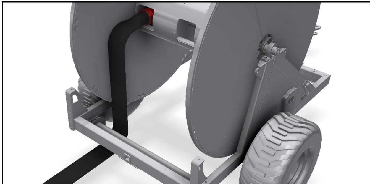
Figure 16 - Insert Hose into Reel Opening
